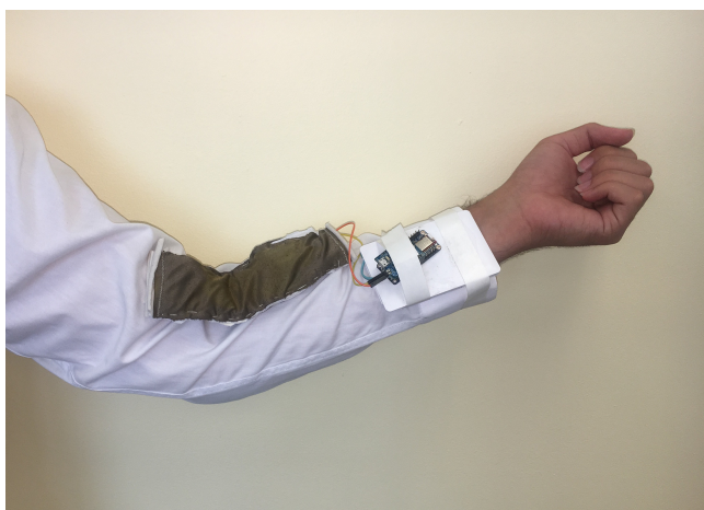
Figure 10: User wearing Tribexor implemented as a sleeve.
